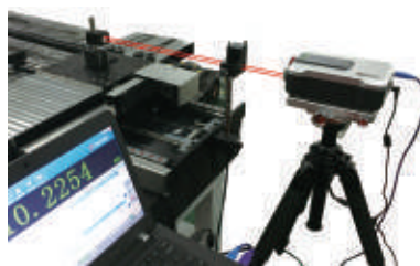
Linear meas. of stage module
