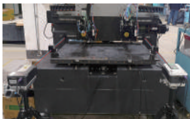
Twin guide rails meas. of equipment
