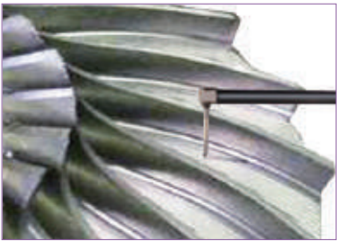
Ra of engine blade
