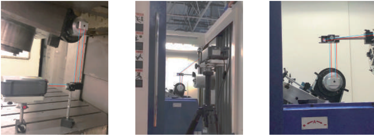
Eccentric axis measurement
