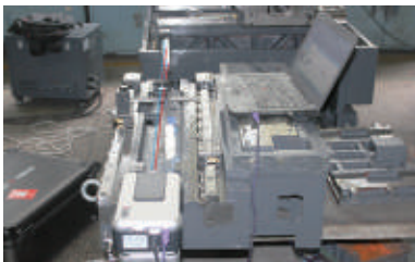
Parallelism meas. of two guide rails
