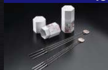
ねじ測定用三針ゲージ 3-wire gauge for measuring threads
