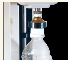
PET bottle compression strength test with PC-5060.
