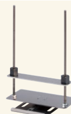
Opening testing for pull-tab of canned food's container.
