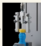
Cap Tension test with SHF-100N
