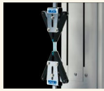
Rubber tension strength test with PGC-0510.
