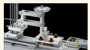
Coefficient of friction test for lipstick&artificial skin
