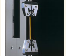
Cable tension strength test with KC-1001.
