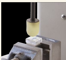
The switch tactile test with UR-8S.
