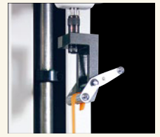
Rubber tape tension strength test with GC-60.
