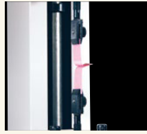
180 degree peel testing of adhesive tapes with FC-21
