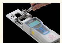
Pinching strength test of forceps with PCA-150N
