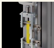
PP band tension strength test with PPC-5000N.
