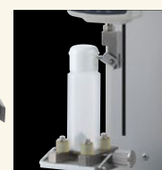
Flip Cap Opening test with HFC-50N
