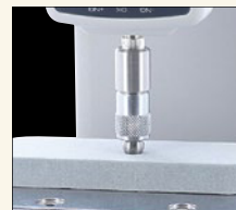
Hardness test of cushioning material with SP-5010
