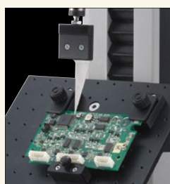
Endurance test for surface mount solder joint with SJ-QFP-01.
