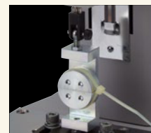
Binding band tension strength test with LOP-1000N
