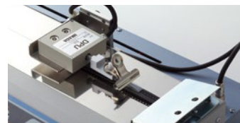
Peel test of embossed carrier tape
