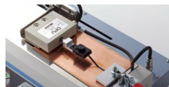
Peel test of copper foil
