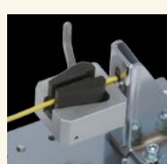
Cable tension strength test with CW-500N.
