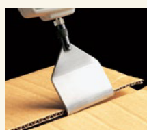
Corrugated card board opening strength test with DF-60
