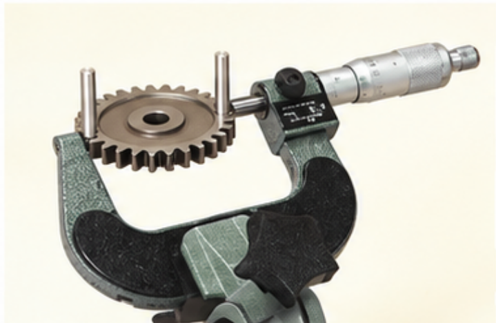
Measuring Over Pin Diameter of Gear
