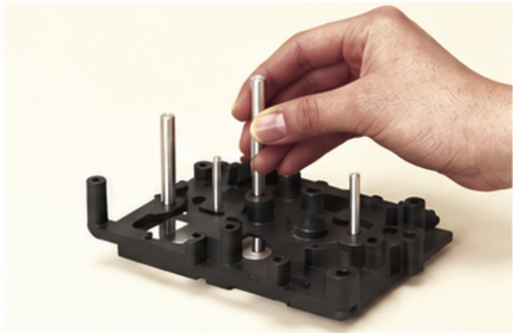
Checking hole Diameter
