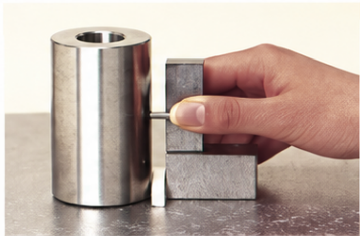
Checking Right Angle
