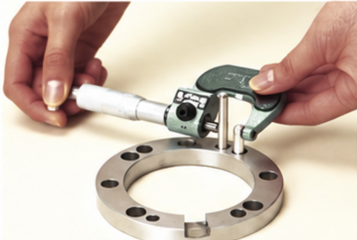
Measuring Distance Between holes
