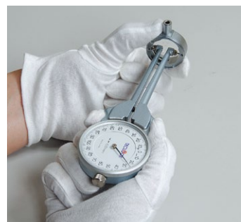
Measuring example of inner diameter of a small metal work piece.
