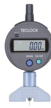
DMD-252S2 φ3.2 Steel Ball Contact Point Resolution 0.01mm Measuring Range Concave 5mm Convex 4mm
