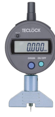
DMD-2520S2 φ3.2 Steel Ball Contact Point Resolution 0.001mm Measuring Range Concave 5mm Convex 4mm
