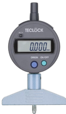
DMD-2130S2 φ3.2 Steel Ball Contact Point Resolution 0.001mm Measuring Range 10mm
