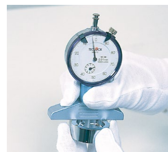
Measuring depth of concavity of work of which center is bored. The photo shows 2.03mm.
