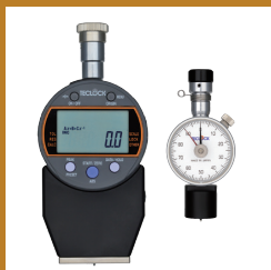
Pocket type and Digital Durometer with peak hold type.
